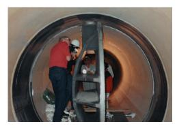
FLEXICLAD® DuraTough™ DL is a two component, 100% solids, fluid consistency elasto-ceramic polymer composite specifically formulated to surface and protect equipment subject to cavitation accelerated erosion/corrosion.
